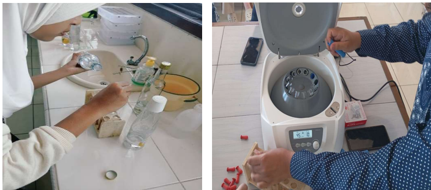
Figure 3. Nanoplastic Precipitation Process Using a Centrifuge
